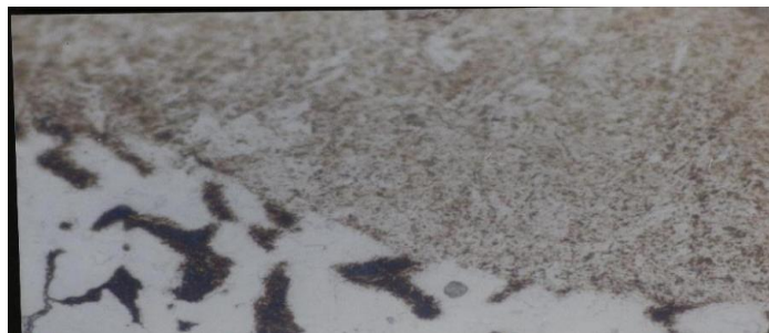
Figure2. General view of laser surface melted region of carbon steel, 500X. (Laser power 90W, Scanning velocity 1.00mm/s)
